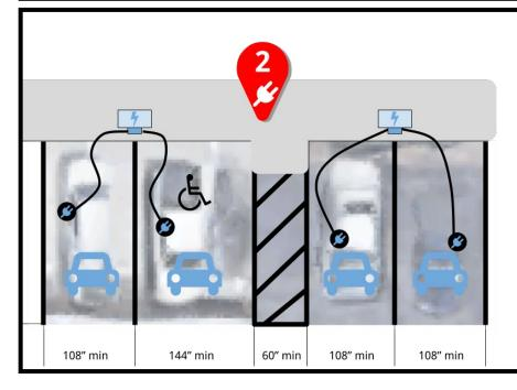
In this configuration, the charging stations are on the sidewalk. The sidewalk must be at least 48 inches of unimpeded space.
